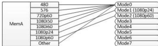
Figure 2, Input memories linked to different output memories
