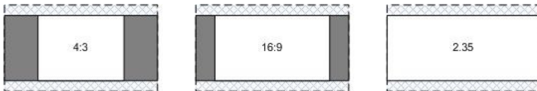
Figure 1, 16:9 projector with fixed zoom used on a 2.35 screen
