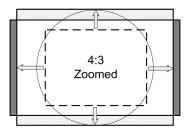
The Radiance has a "NLS" setting, to correctly stretch Windowboxed 4:3 video for a 16:9 display. Different "NLS" settings can be made to each input. The "NLS" setting is stored in the user memory under "MemX->Input->Resolution->Size (aspect)".
