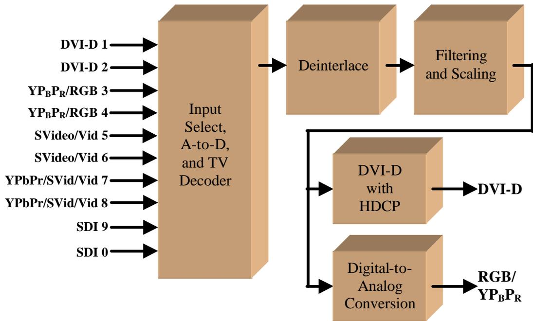
VisionPro HDP Functional Block Diagram
